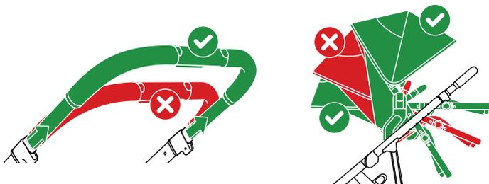
Use only with the handlebar fully extended when the toddler seat is in the rear-facing position.
